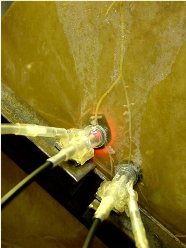
Fig. 1. Single-nodule chambers, applied here to alfalfa (*Medicago sativa*) roots, allow experimental control of  $N_2$  fixation by varying  $N_2$  concentration. An optical fiber touching the nodule surface monitors transmission of red light through the nodule, which depends on the oxygenation status of the leghemoglobin inside.
